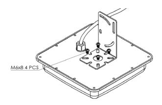
Step 2: Take off the nuts and gaskets from U-bracket. Set the U-bracket into any cylinder at the site. Gradually attach the Fixed Bracket and Step 1 to U-Bracket and fixed by the nuts and gasket.
