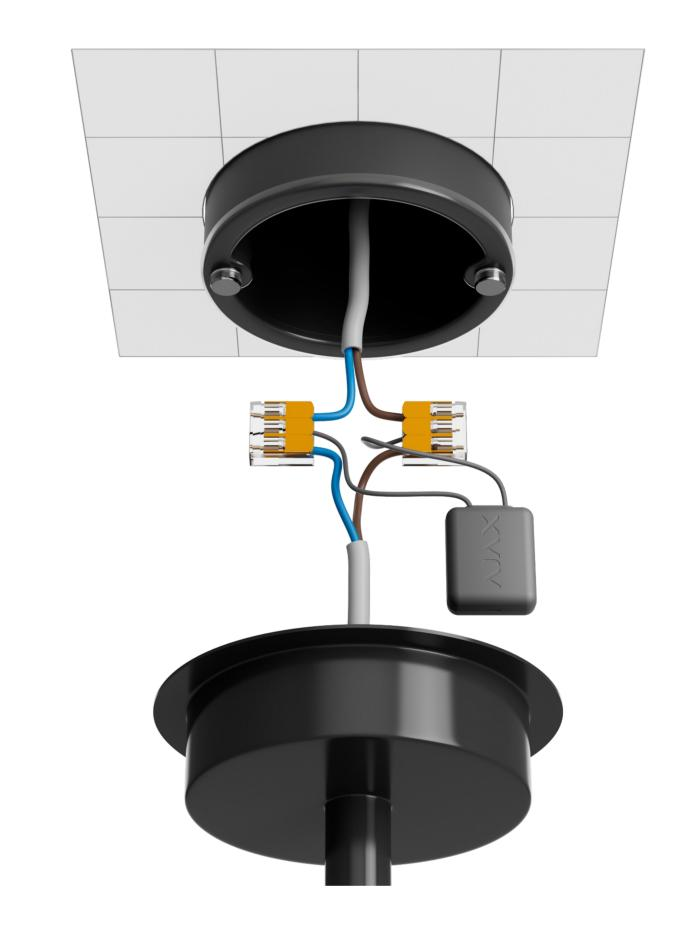
Bypass (Dimmer) [55] does not connect to the hub and therefore is not displayed in Ajax apps.
