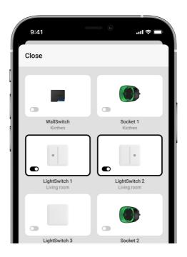
The lighting also can be controlled in the **Control** • menu. To do this, go to the **Control** • menu and swipe up. All control devices added to the hub will appear in the list. Click on the switch in **LightSwitch** field, and the state of the device's contacts will change to the opposite. The lighting will switch on or off.
