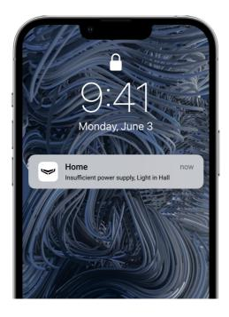
LightSwitch regularly measures the switching current. If LightSwitch controls the power of a lighting device with insufficient power (up to 5 W), the system will notify the users of the Ajax system. In this case, it is necessary to replace the lighting device with a similar one with higher capacity or to connect a bundled capacitor in parallel with the lighting device.
