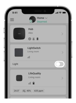
Press the switch in **LightSwitch** field in the **Devices** menu in the Ajax app, and the state of the switch contacts will change to the opposite; lighting will be switched off or on. This way, system users can remotely control the lighting. For example, switch on the light in the room in advance before entering the room.
