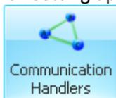
From the **Communication Handlers** panel, disable and restart the Modbus service to cause it to load the new mapping data. The service must be restarted whenever new Modbus mapping addresses are configured or imported in order for the service to reload the mapping data.
