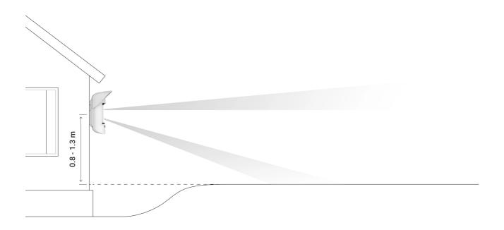
**The detector can be placed 0.5 meters above ground level** to protect the facility from crawling burglars. In this case of installation, the pet immunity function is not available. This mounting height of the detector is recommended for installation in industrial facilities and warehouses.
