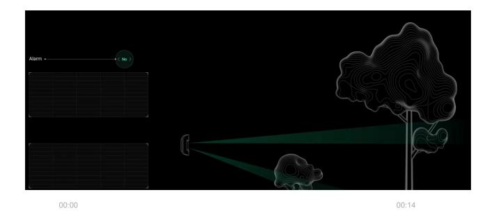
MotionCam Outdoor features two independent IR sensors, the signals of which are analyzed by a two-stage LISA algorithm. As soon as both IR sensors detect movement, LISA performs correlation and spectral analysis of the signals, which allows you to instantly distinguish between real threats and interference.
