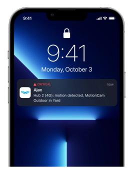
Users know exactly where motion is detected. The notifications contain the name of the hub (name of the guarded object), the name of the device, and the virtual room to which the detector is assigned.
