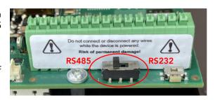
Please connect the RS485 or RS232 serial lines directly from TBS device to controller:
