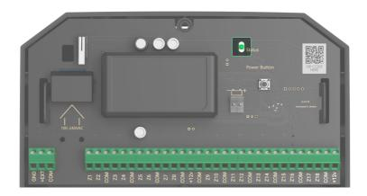
The MultiTransmitter LED indicator may light up in white, red, or green depending on the device status. Note that the LED indicator is not visible if the lid is closed, but you can check the device status in the Ajax app.
